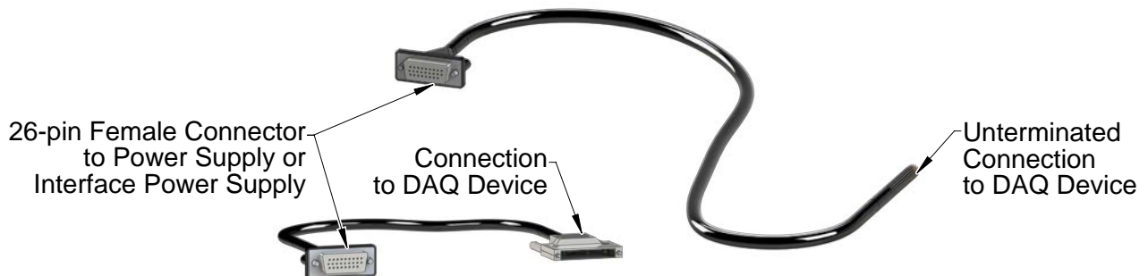
Figure 2.8—Power Supply Cables
