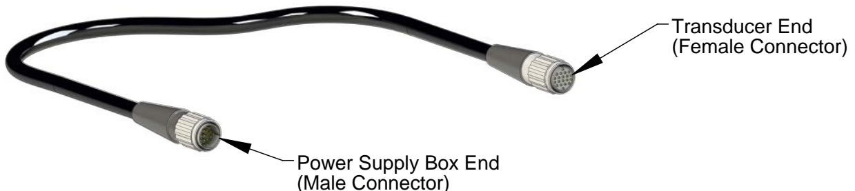
Figure 2.5—Transducer Cable for 9105-TIF Transducers
